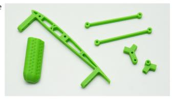
2. Shell parts (wings). Use 0% infill and no horizontal surfaces (thickness of the shell is one layer). Only this way you can achieve required weight of the plane.
