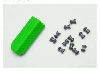
Remove the nose from the fuselage. Insert 12 airgun pellets (177 Cal) into it and secure the pellets in place with the glue.
