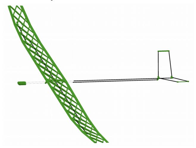
Slide the wing onto the fuse spars. Then insert the nose back onto the fuse spars and secure it with the glue. Leading edge of the wing should be 10,3 cm from the end of the nose.
