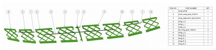
Assembly the wing as sketched above. Hold on to the order of the parts as indicated in the picture.
