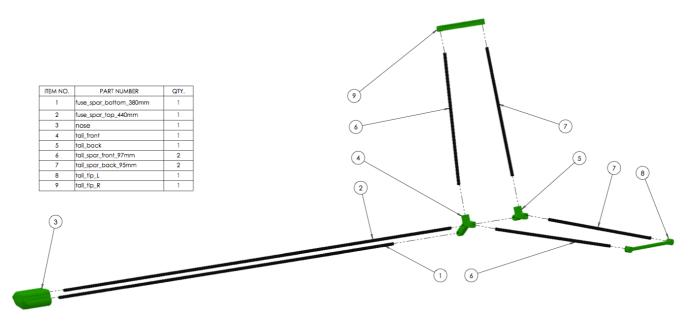
When assembling the fuselage start with the nose and both fuse spars, but **do not glue it** yet. Nose helps to align the spars during assembly and has to be removable so that during final assembly the wing can be slide on to the fuse spars. Build the rest of the fuselage as sketched above.
