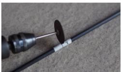
TIP: Carbon wing joiner tubes on the fuselage should fit into spars in the wing. Sometimes the fit is too tight or you cannot insert joiner tubes into wing spars at all. You can use drill and wet sandpaper to make joiner tubes thinner. Use breathing mask to avoid inhaling carbon dust!
