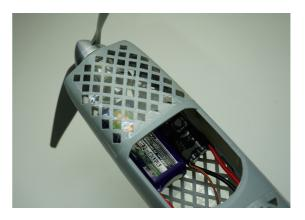
Although there is plenty of space in the fuselage, to be able to set correct CG, you have to place ESC and Battery next to each other right behind the motor. In this configuration ideal battery weight is between 120g and 140g. *Turnigy nano-tech 1500mah 3S 25~50C Lipo Pack* is one of many options.
