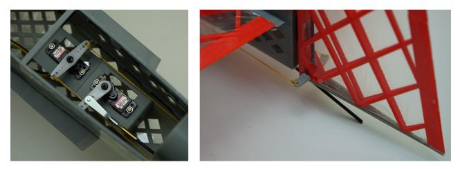
Rudder has pull pull system as shown on the pictures above.
