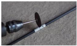
TIP: Joiner rods on the fuselage have diameter of 4 mm, carbon spars in wings have inner diameter of 4 mm. They should fit into each other but sometimes the fit is too tight or you cannot insert joiners rods into wing spars at all. You can use drill and wet sandpaper to make joiner rods thinner. Use breathing mask to avoid inhaling carbon dust!
