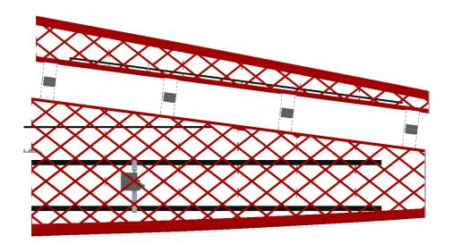
Some hinge slots are not deep enough to fit whole hinge length. Shorten all hinges as shown on the picture. It has no benefit in terms of added stiffness of rigidity to use whole hinge arm length as only small hinge area is in contact with the wing.
