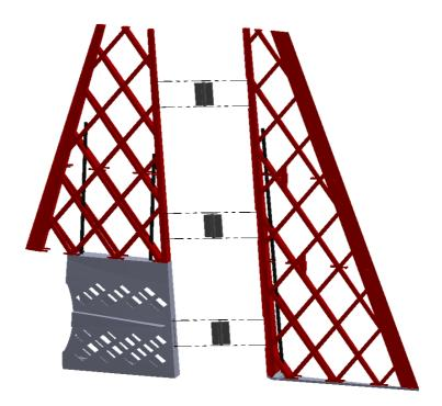
To complete vertical stabilizer assembly first shorten all hinges and then insert the hinges into hinge slots and apply the glue from inner side of the main part. Then insert all hinges into hinge slots on moving part and put the glue from inner side of the moving part.
